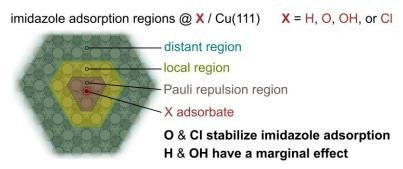
Figure 1. Three different adsorption regions of imidazole on X/Cu(111) with respect to its lateral distance to X(ads).
