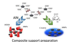
Figure 1. A schematic representation of composite support preparation from MNPs. The precursors require further processing.
