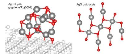
Figure 1. Structural comparison between  $Ag_{11}O_{12}$  cluster (left) and AgO bulk oxide (right). The hybrid structure composed of Ag(I) and Ag(III) ions bounded to two and four O atoms and the related local AgO<sub>4</sub> configuration of AgO is preserved in the cluster.
