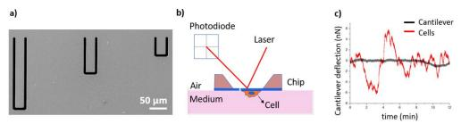
Figure 1. a) SEM image of the rectangular cantilevers separated from the membrane by a groove; b) scheme of the PWMD setup; c) example of a the deflection curve as function of time for bare cantilever (black) and in presence of MDA-MB 231 cells (red) recorded in PW conditions.
