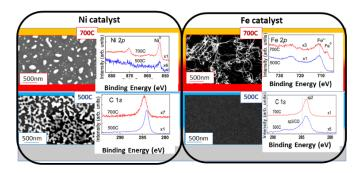
Figure 1: SEM images and relative XPS spectra of C-NSs synthetized using different catalysts (Ni, Fe) and CVD temperatures (500C, 700C). The used CVD precursor gasses were C2H2 (100sccm) and H2 (100sccm) and the processes duration was 5-10 min.
