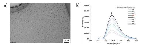
Figure 1. TEM image (a) and FL spectra (b) of B, N-doped GQDs obtained from citric acid, boric acid, and urea under microwave irradiation.
