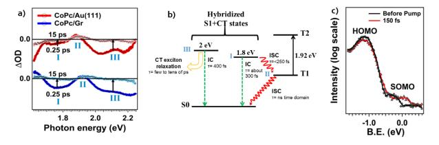
Figure 1: a) CoPc/Gr and CoPc/Au(111) TAS spectra in the Q-Band energy region; b) Jablonski diagram of the relaxation channels in the CoPc thin film ( $\tau$ = decay time, So/1 = singlet state, T1/2= triplet state, IC= internal conversion, ISC= intersystem crossing); c) CoPc/Au(111) sample TR-PES spectra before and after the 2 eV pump pulse.
