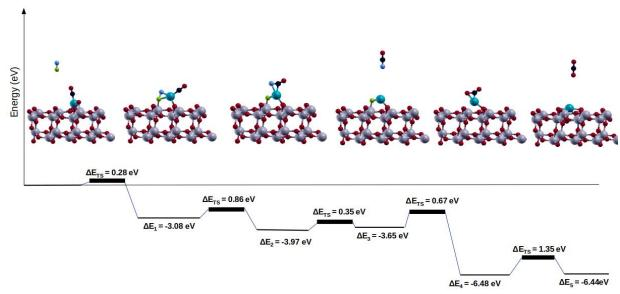
Figure 1. Full catalytic cycle of CO oxidation on TiO<sub>2</sub> supported single Pt atom.
