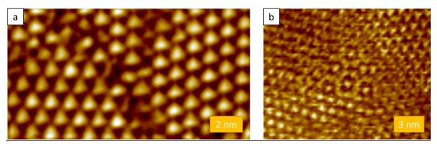
Figure 1. a) Left- and right-handed domains in 1T-TaS2 with a domain wall in-between. b) "Flower-shaped" patterns (in the center) of two-chirality interference in the region of L and R coexistence.
