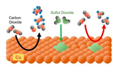
Figure 1.  $CO_2$  reduction on copper can be affected by the reaction of the surface with sulfur dioxide to change its selectivity. Reprinted with permission from reference 2. Copyright 2021 American Chemical Society.
