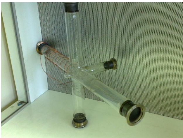
Figure 30: Glow discharge chamber . Borosilicate glass Schott 8250.
