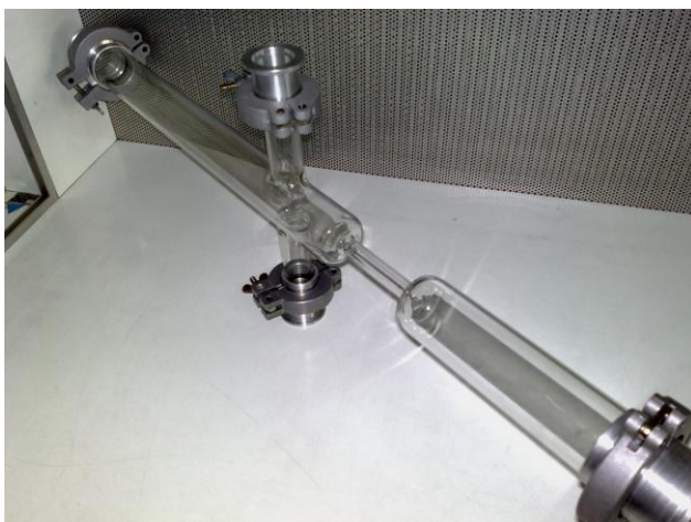
Figure 31: Afterglow chamber . Borosilicate glass Schott 8250.
