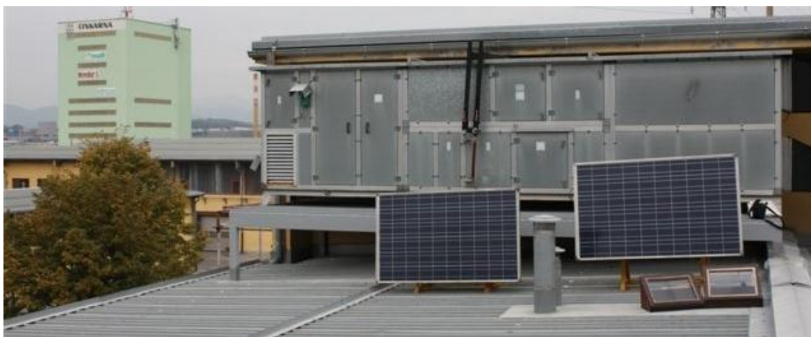
Figure 55: Si solar modules and glass substrates that were used to determine the photocatalytic activity of the coatings.
