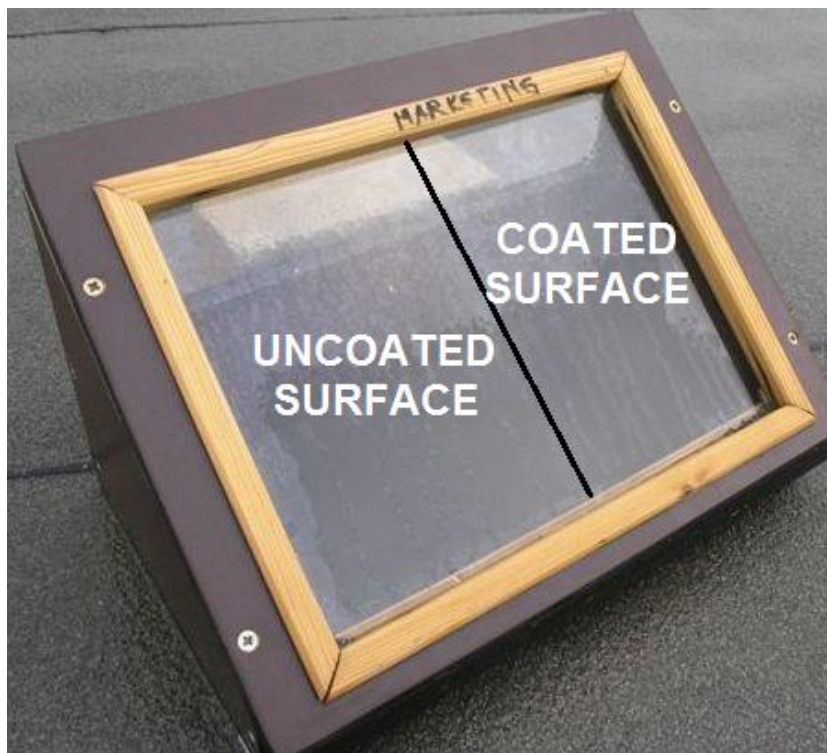
Figure 64: Glass surface after two months exposure to real-life environmental conditions. The PSH effect of the coated side is not observable. The coated and the uncoated side of the glass substrate look almost the same.
