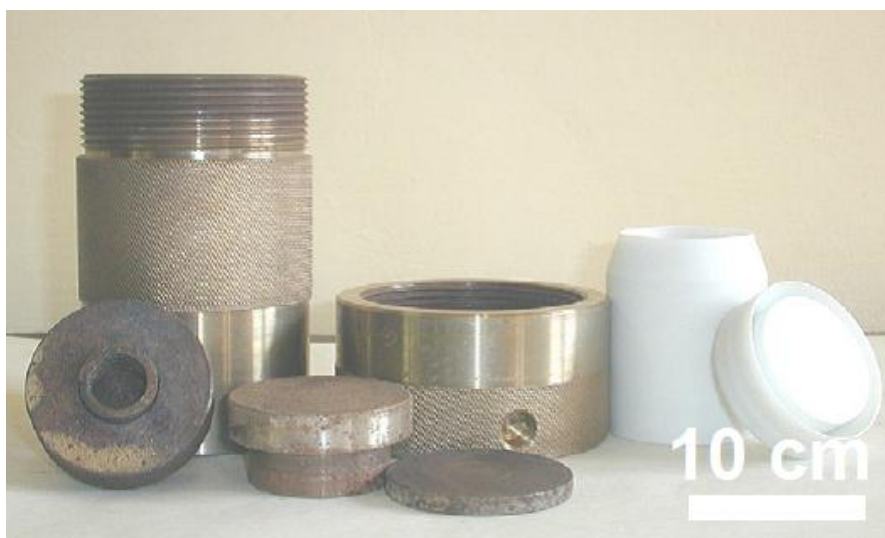
Figure 6: A typical autoclave used for laboratory hydrothermal synthesis experiments.
