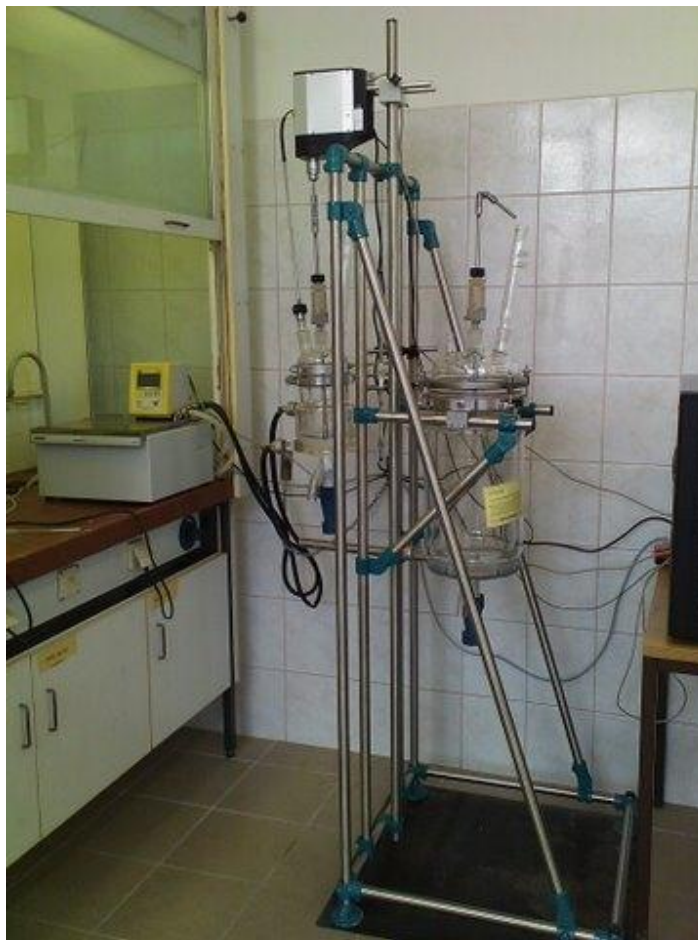
Figure 14: The reactor system set up in Cinkarna Celje laboratory used to carry out the sol-gel and gel-sol synthesis reactions.
