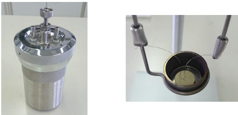
Figure 3.2: Oxygen combustion bomb (left) and combustion capsule with sample pellet and a wire between two electrodes (right).
