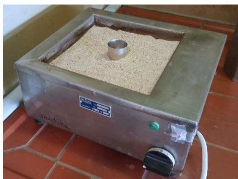
Figure 3.1: Evaporation on a sand bath (left) and fusion with Na_2CO_3 (right).
