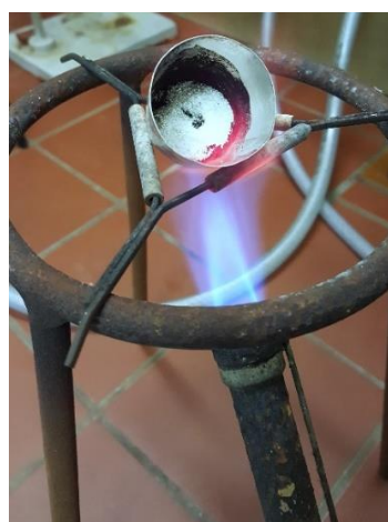
Figure 3.1: Evaporation on a sand bath (left) and fusion with Na_2CO_3 (right).
