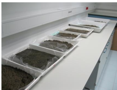
Figure 3.10: Drying of sediment samples. Photo: Urška Remic.
