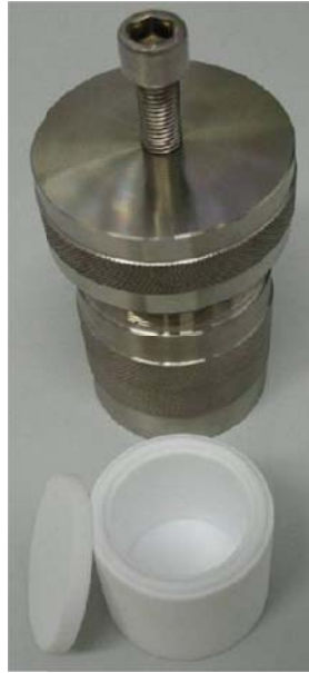
Figure 1: Example of an autoclave with a Teflon vessel.
