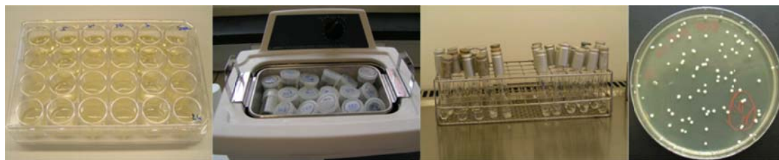
Figure 7: Procedure for biofilm formation test. From left to right; Incubation of bacteria with BAG pellets, detaching of bacteria from pellets surfaces, serial dilutions and bacteria colonies on agar plates after overnight incubation.
