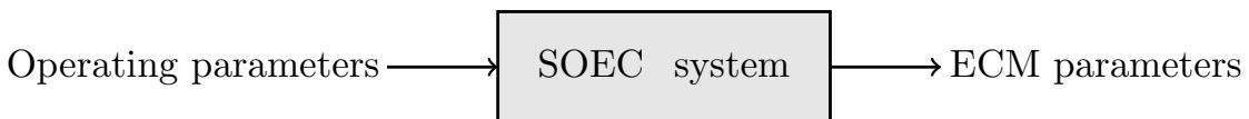
Figure 3.2: The idea of modelling the equivalent circuit model parameters \theta_i, i = 1, \dots, m as a function of the vector of process variables \mathbf{x} .
