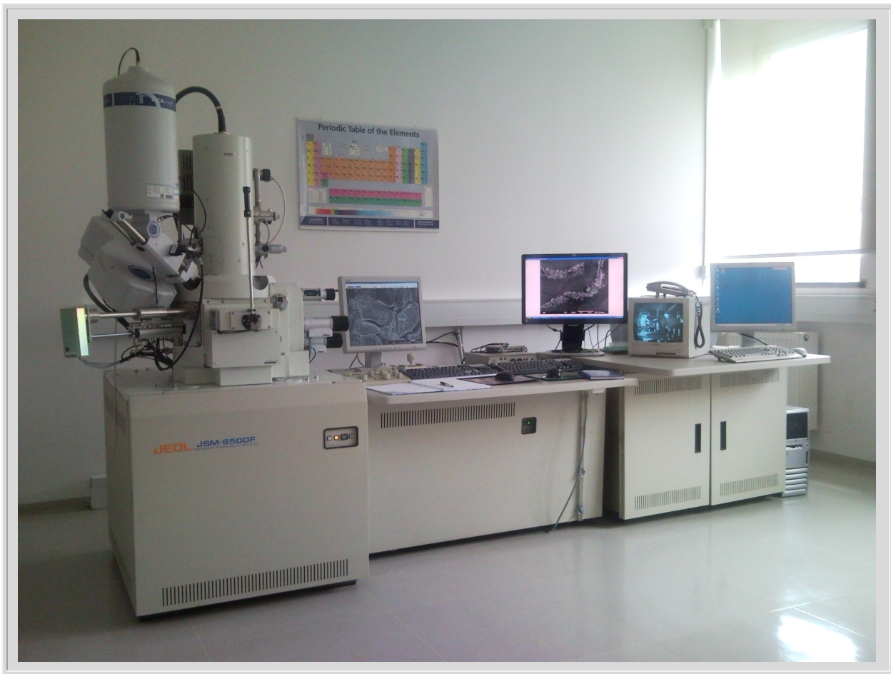
Figure 5: Field Emission Scanning Electron Microscope JEOL JMS- 6500 F (manufactured JEOL Ltd. Japan) Institute of Metals and Technology, Ljubljana.
