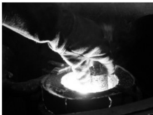
Figure 4: Charging of compact into melt Slika 4: Dodajanje stisnjencev v talino
