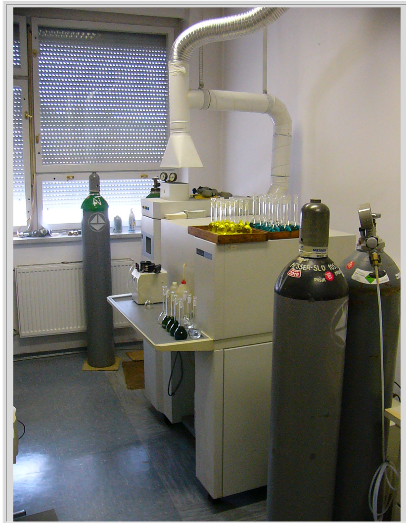
Figure 8: Inductively coupled plasma optical emission spectrometry (ICP-OES), model: PERKINELMER Optima 3100 RL (IMT, Laboratory for chemistry)
