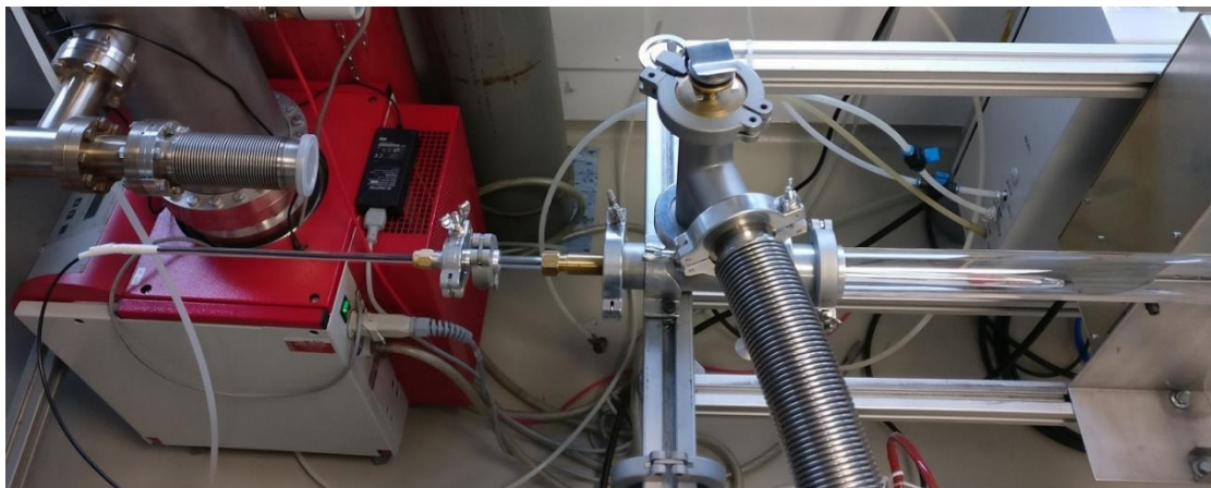
Figure 2.7: Catalytic probe. Shown mounted onto the pilot-scale plasma system for measurements during treatment of cloves in the H-mode afterglow.
