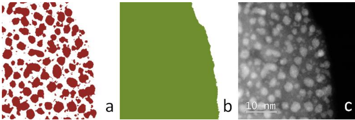
Figure B.13: STEM-HAADF images of the two-phase nanocomposite CTiON-NCNF1 which consists of the C matrix and TiON nanoparticles. (a) the outline of the TiON nanoparticles made with three steps: Gaussian blur, rolling ball background subtraction, and thresholding. (b) the outline of the CTiON-NCNF1 area was made with two steps: Gaussian blur and thresholding. (c) the original image. To estimate the nanopore volume fraction, a separate image was used.
