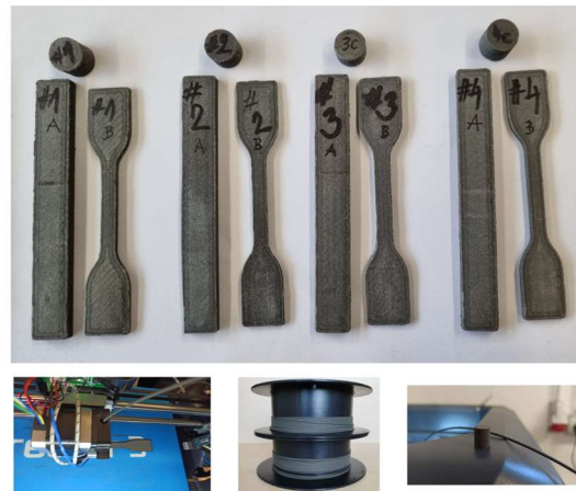
Figure 5-2: Images of FDM printed tensile, flexural test samples, and cylinders (a), FDM printing of tensile test sample (b), extruded and spooled filaments (c), and FDM printed cylindrical magnet (d).
