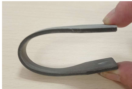
Figure 4-8: Dog-bone-shaped specimen, FDM-printed from filament S90/10, fully bent without breaking.
