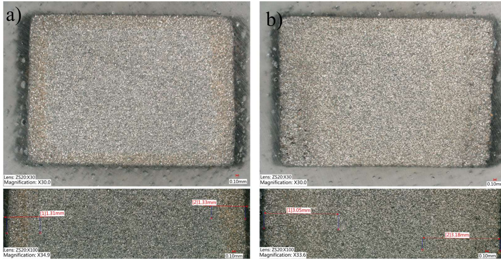
Figure 4-13: Surface corrosion, cross-section microscopic images of magnets S90/10 (a) and B90/10 (b) showing progress of corrosion after immersion in corrosive water at 95 °C for 1000 h.
