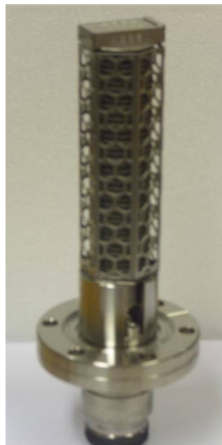
Figure 11: Photograph of the SAES Getters CapaciTorr pump models that use a 2 1/2" Conflat flange. The D-400 cartridge uses St 172 (Zr-V-Fe) getter alloy. CapaciTorr pumps use porous sintered getter elements in the cartridge
