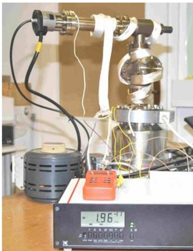
Figure 68: A system for testing ultimate pressure of turbo pump TMP1
