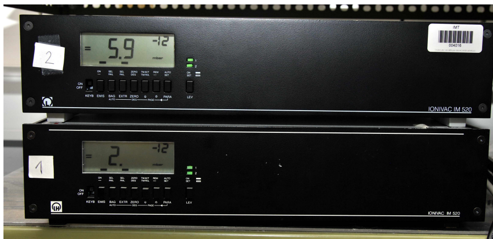
Figure 78: Photo of extractor gauge readings at ultimate pressure.
