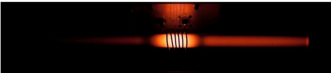
Figure 1.55. A photo of the discharge tube when nitrogen plasma is in the H-mode, i.e. at 40 Pa and 500 W forward power.
