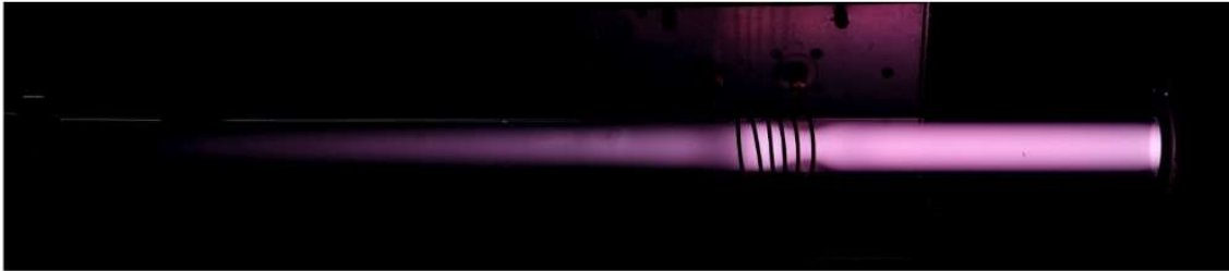
Figure 1.44. A photo of the discharge tube when hydrogen plasma is in the E-mode, i.e. at 20 Pa and 150 W forward power.
