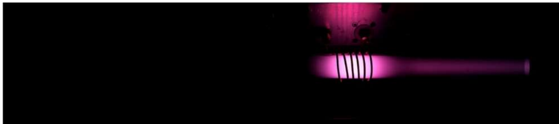
Figure 1.45. A photo of the discharge tube when hydrogen plasma is in the H-mode, i.e. at 20 Pa and 500 W forward power.
