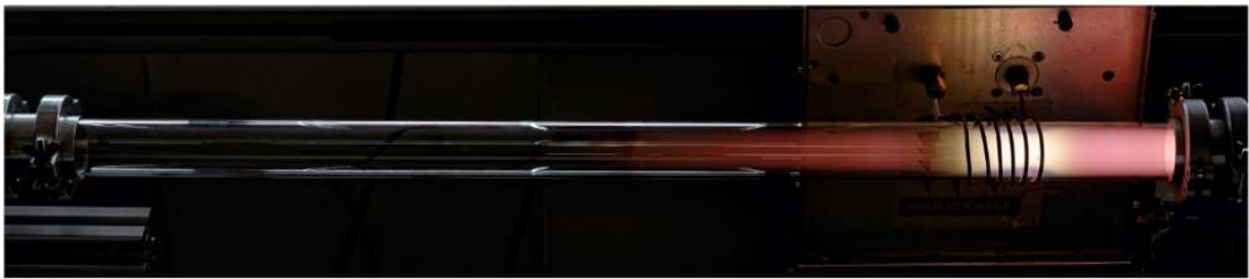
Figure 1.33. A photo of the discharge tube when oxygen plasma is in the E-mode.
