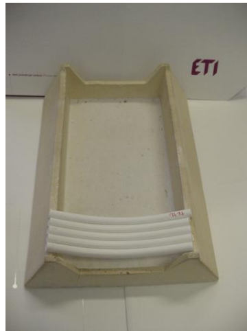
Figure 3.5-1. Refractory saggar with deformed samples after firing in gas kiln.
