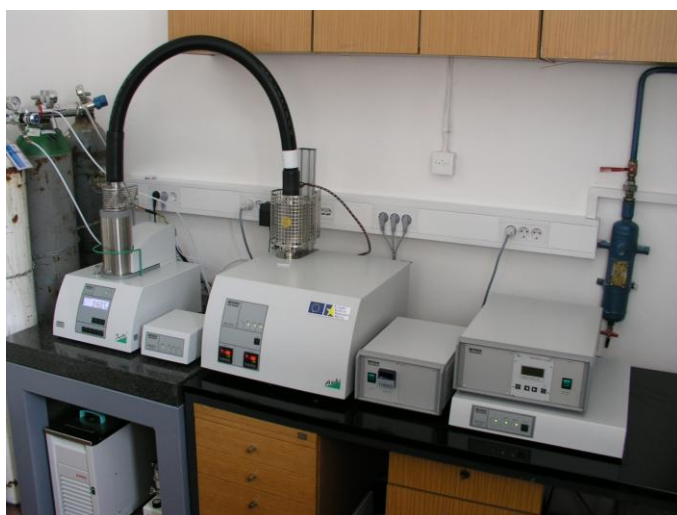
Figure 30: TG-DTA/DSC with Gas Analytical System QMS 403 C Aëolos (STA 449 C/6/G Jupiter® - QMS 403 C, Netzsch, Germany) thermal analyzer with attached mass-spectrometer. On the right, corresponding schematics is shown.
