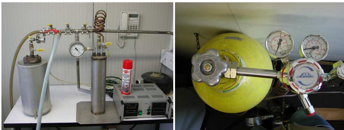
Figure 22: Photography of our stainless-steel Sievert's apparatus for high-pressure hydrogen absorption.
