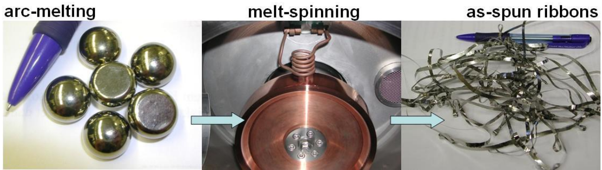
Figure 19: Processing route of melt-spun ribbons.
