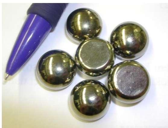
Figure 24: Arc-melted buttons of Ti-Zr-Ni alloys. Each weights about 5 grams.
