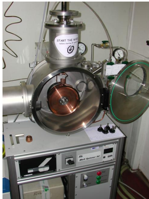
Figure 20: Edmund Bühler, Melt Spinner SC device.
