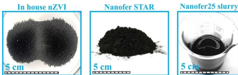
Figure 3.5: In-house nZVI in suspension and collected over a magnet, Nanofer STAR powder, and Nanofer25 slurry in a beaker.
