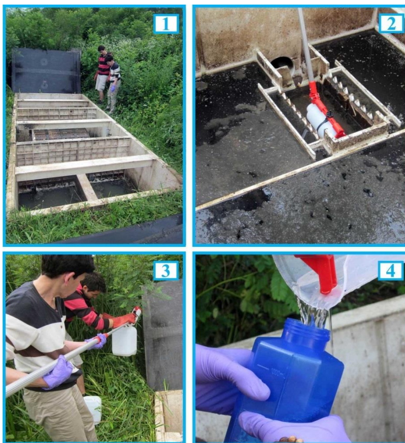
Figure 3.4: The SBWTP Hruševo (1) with its top open; sample is taken with a telescopic swing swivel dipper at the outflow (2) and transferred in sterile plastic containers (3) and (4).
