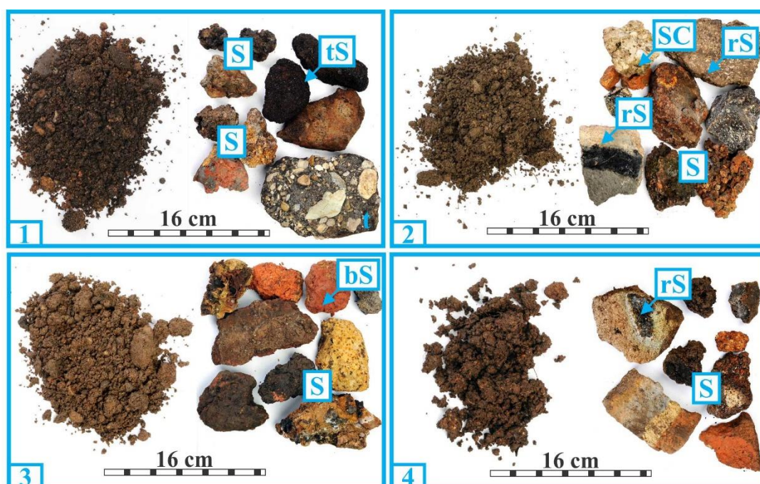
Figure 5.1: Representative CS samples and larger pieces of material from the sampling area one (1), two (2), three (3) and four (4) from the Old Zinc-works site. Larger pieces of slag (S), tar-impregnated slag (tS), refractory materials impregnated with slag (rS), concrete with slag (SC), and brick with slag (bS) are also presented.
