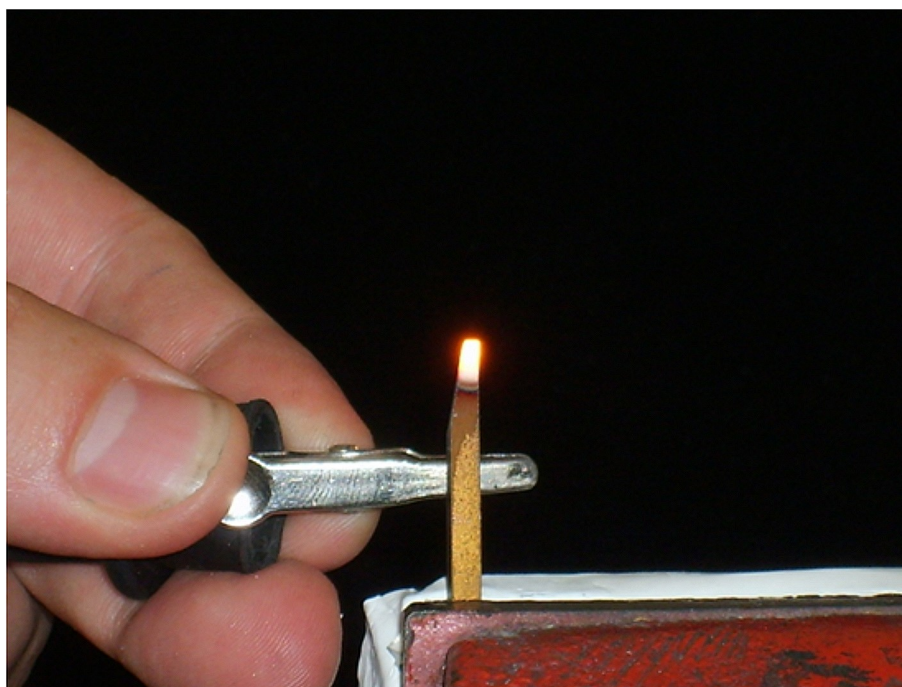
Figure 79: Glowing of the designed prototype at 1300 °C.
