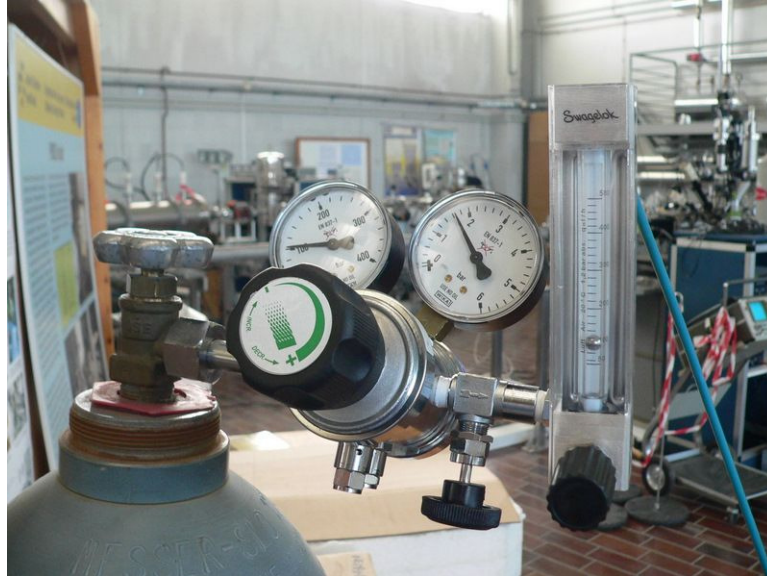
Figure 10: A flow-meter with precision needle valve at external beamline at Microanalytical center at Jožef Stefan Institute. The flow-meter is necessary to ensure the constant flow of helium gas to the target.
