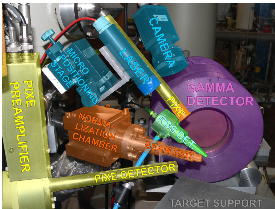
Figure 31: The external beam experimental setup at Microanalytical center at Jožef Stefan Institute with the PIXE, PIGE and RBS detectors. Normalization chamber with the wire-mesh-based charge-collecting device is seen, as well as the positioning system with a camera and a laser fixed on a micro-positioning stage.
