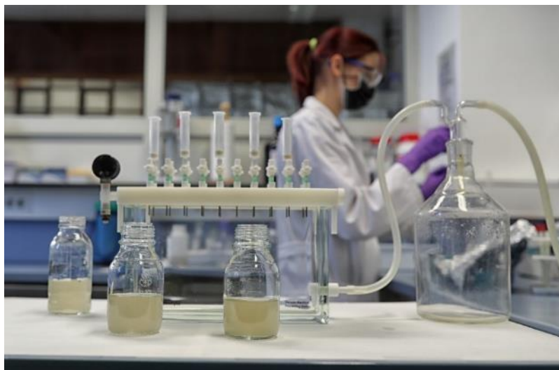
Figure 6: SPE manifold with extraction cartridges and wastewater samples (Photo: Blaž Samec).
