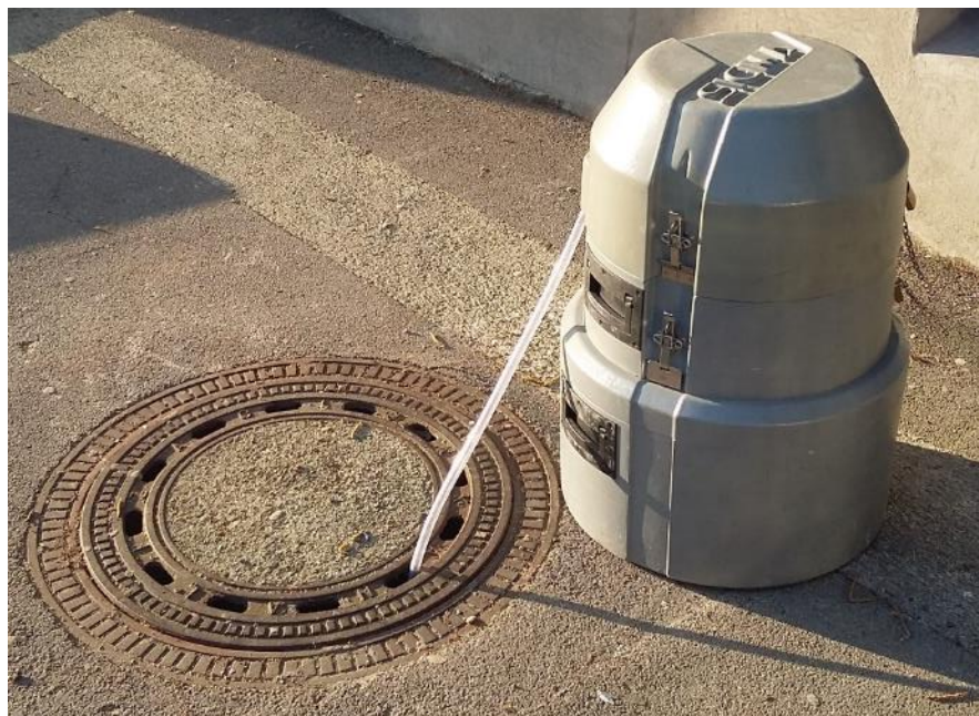
Figure 4: Example of sampling wastewater in specific sub-catchment using autosampler (Photo: Taja Verovšek).
