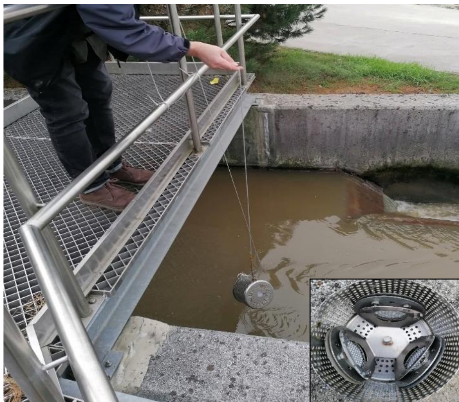
Figure 3: Setting passive sampler (POCIS) at municipal WWTP (Photo: Taja Verovšek).
