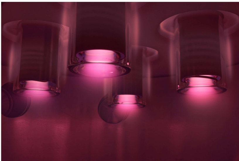
Fig. 4. A photograph of the four ICPs in the plasma reactor at 20 Pa and real power of 1800 W.
