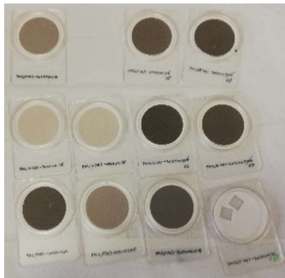
Figure 3: PM collected on quartz fiber filters in different seasons.
