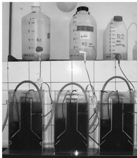
Fig. 2 Experimental set-up of the three pilot WWTP reactors (R0, control; R1 and R2, 0.05 and 0.005 \text{ mg L}^{-1} , respectively, of the pharmaceutical mixture)
