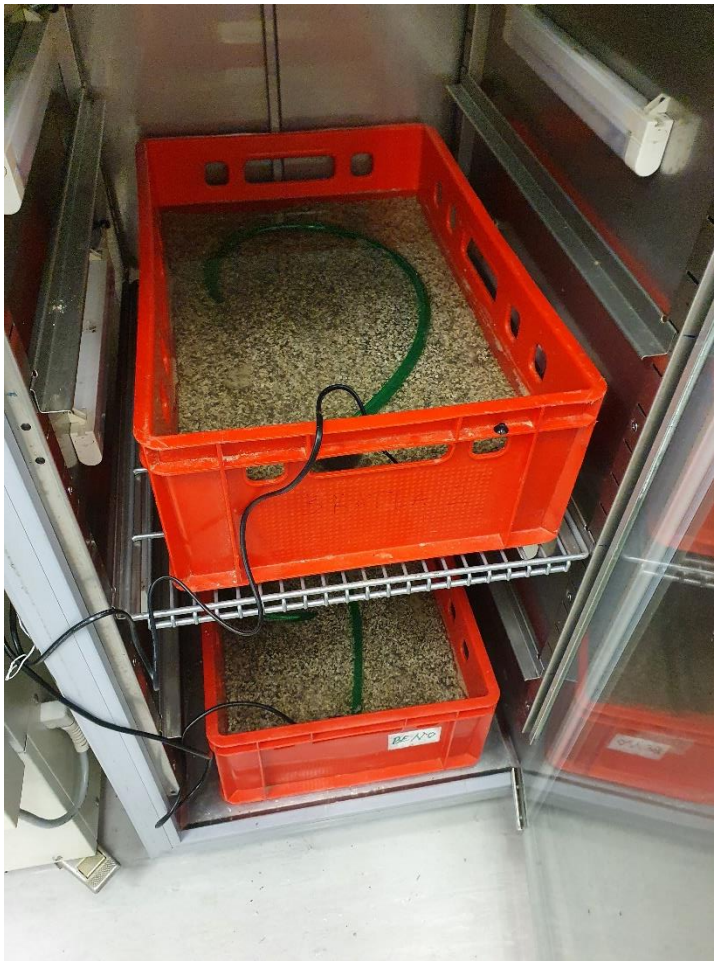
Figure 35: The containers with the incubated sediments. On top of sediment the green tubes, connected to water pump are visible.
