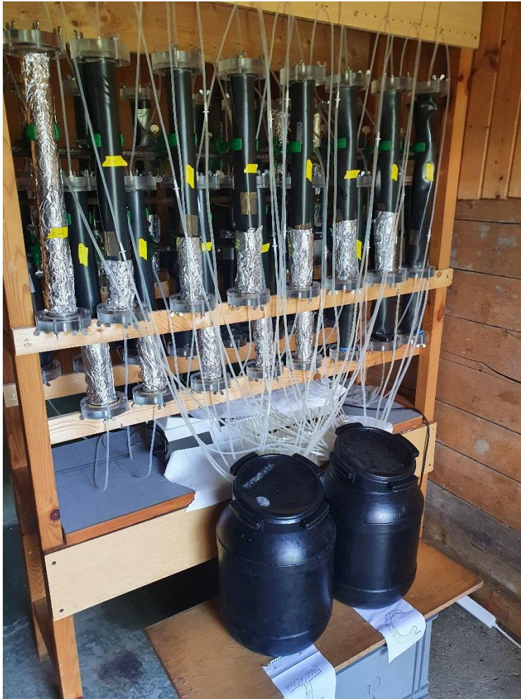
Figure 36: Photo showing the mesocosm experimental setup, with covered and upright reactors connected to separate water tanks (control and treatment).
