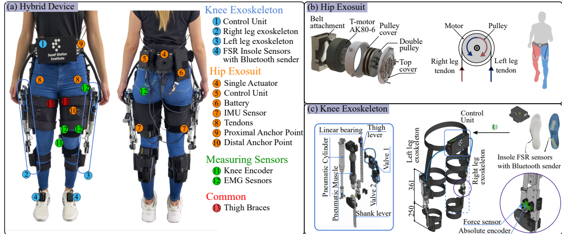
Figure 6.1: (a) Overview of the hybrid exoskeleton with labeled parts. In (b) hip exosuit features a tendon-driven actuation with a double-layered pulley, where each layer contains a tendon so that one direction of motor rotation assists one leg and vice versa assists the other leg. In (c) knee exoskeleton comprises three main parts: the control unit, the left leg, and the right leg exoskeleton. The actuator includes a pneumatic cylinder, pneumatic muscle and two air solenoid valves. Compressed air is supplied from the air compressor. Insoles with FSR sensors inside shoes wirelessly transmit signals to the control unit.
