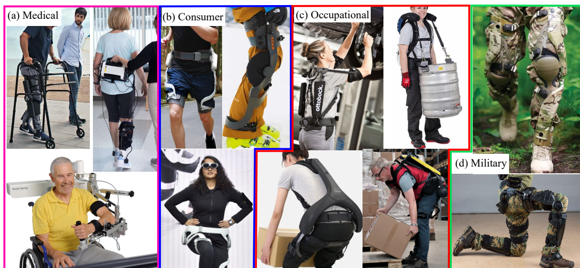
Figure 1.1: (a) Medical: ABLE by ABLE Human Motion (lower-limb active exoskeleton), ArmeoSpring by Hocoma (for arm rehabilitation), ReWalk exosuit (for ankle rehabilitation). (b) Consumer: FitExo by Enhanced Robotics, Elevate pneumatic exoskeleton by ROAM Robotics (enhances skiing endurance), GEMS (Gait Enhancing and Motivation System) by Samsung (for haptic feedback in gaming). (c) Occupational: Ottobock Paexo, Atoun by Panasonic, CarrySuit by Auxivo, Cray by German Bionic (enhance endurance during lifting). (d) Military: PowerWalk by Bionic Power, for electrical energy harvesting, and Onyx by Lockheed Martin for increased weight carrying.
