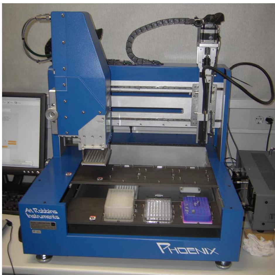
Figure 3: Phoenix pipetting robot. ( http://www.artrobbinsinstruments.com/phoenix.html )
