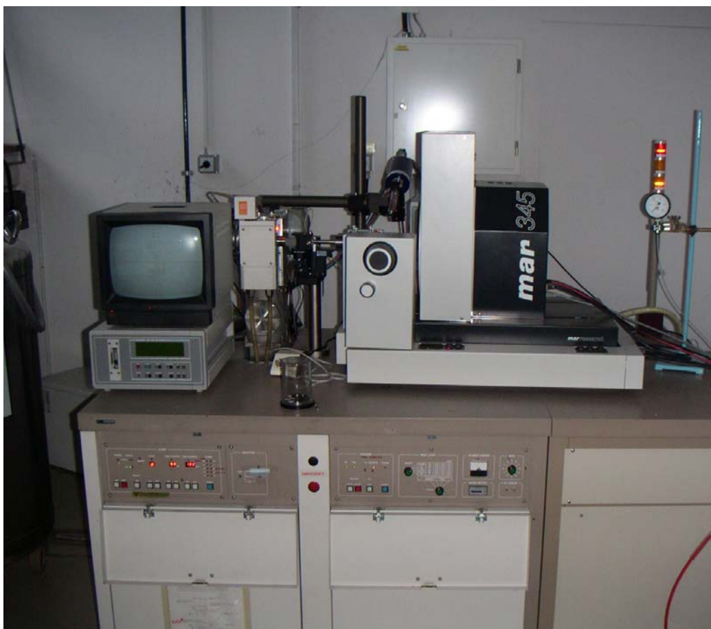
Figure 4: An X-ray source. A Cu-rotating anode X-ray source RU-H2R (Rigaku Corporation, Japan).
