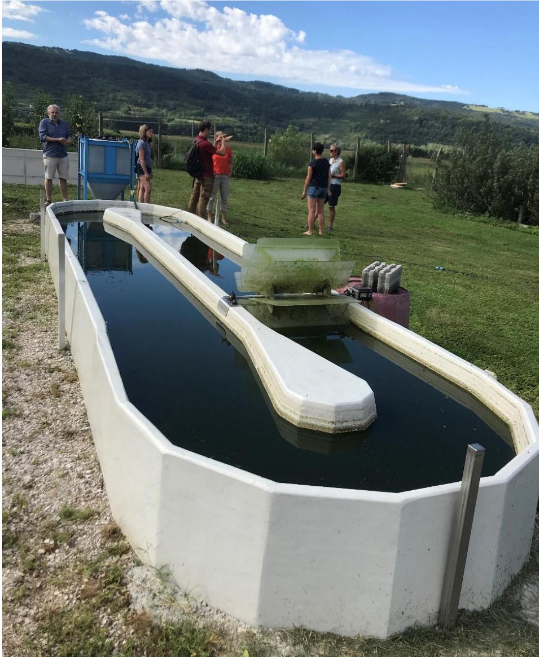
Figure 2: A pilot-scale HRAP in Ajdovščina, Slovenia. (Photo: Ester Heath)
