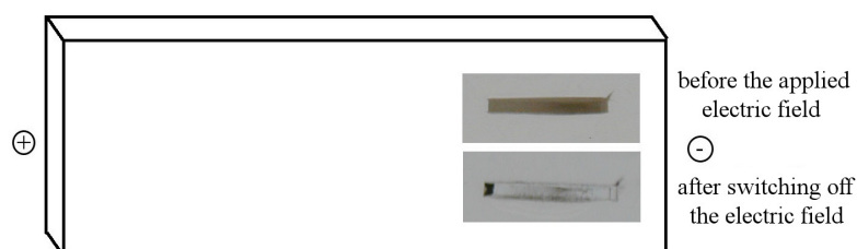
Figure 41: Electrophoresis experiment. Image of the solution in the pocket at the beginning of the experiment (top). In the bottom image, a fraction of the nanowires is deposited on the bottom of the pocket and the other on the vertical wall.
