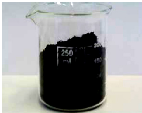
Figure 22: Powder of Mo_6S_{9-x}I_x nanowires. Nanowires collected directly from the ampoule after the synthesis is finished.
