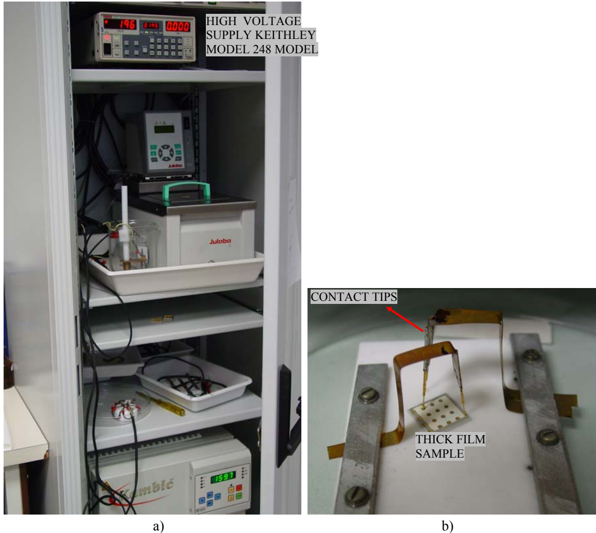
Figure 34: a) The poling setup; high voltage supply KEITHLEY MODEL 248. b) 0.65PMN–0.35P thick-film sample placed on the poling stage between contact tips.
