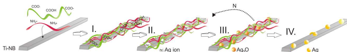
Figure 19: Scheme of the Ag(N)/Ti-NBs composite fabrication procedure.
