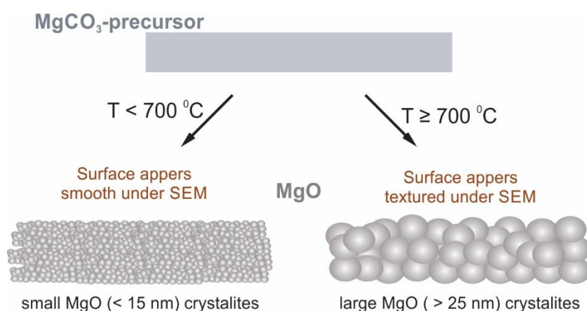
Figure 5. 1: The evolution of nano-texturing at the surface of the MgO microrods.
