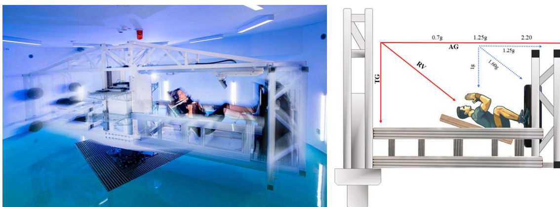
Figure 6: Left panel: European Space Agency (ESA) Short Arm Human Centrifuge (SAHC) in motion (photo credit: K. Bidovec and A. Hodalic). The SAHC has two nacelles. One for the participant and the other for the counterweights. The participant is positioned with the feet on a platform, which can be activated to provide vibration. The unique feature of the SAHC is the sliding gurney on which the subject is positioned. It allows for squats to be performed simulating upright squat exercise. Specifically, the swivel at the centre of mass allows hip flexion and extension during the squat exercise. Right panel: Establishing a ground reaction force of 2.2 g
