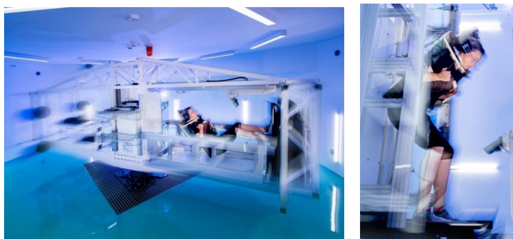
Figure 13: Concept of the short arm human centrifuge (SAHC) is presented in the left panel. It shows the subject lying on the sledge system (same as shown in Fig. 1 above) with the feet on the vibration/force platform. Rotation of the SAHC can establish a gravitational force of up to 4g at the feet. The right panel shows the SAHC in the JSI Gravitational Physiology Laboratory in Planica (Rateče, Slovenia).
