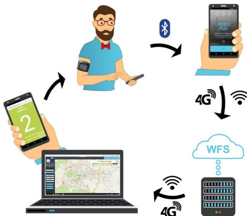
Figure 2. Data flow from the sensor system to the user via a smartphone and the server.
