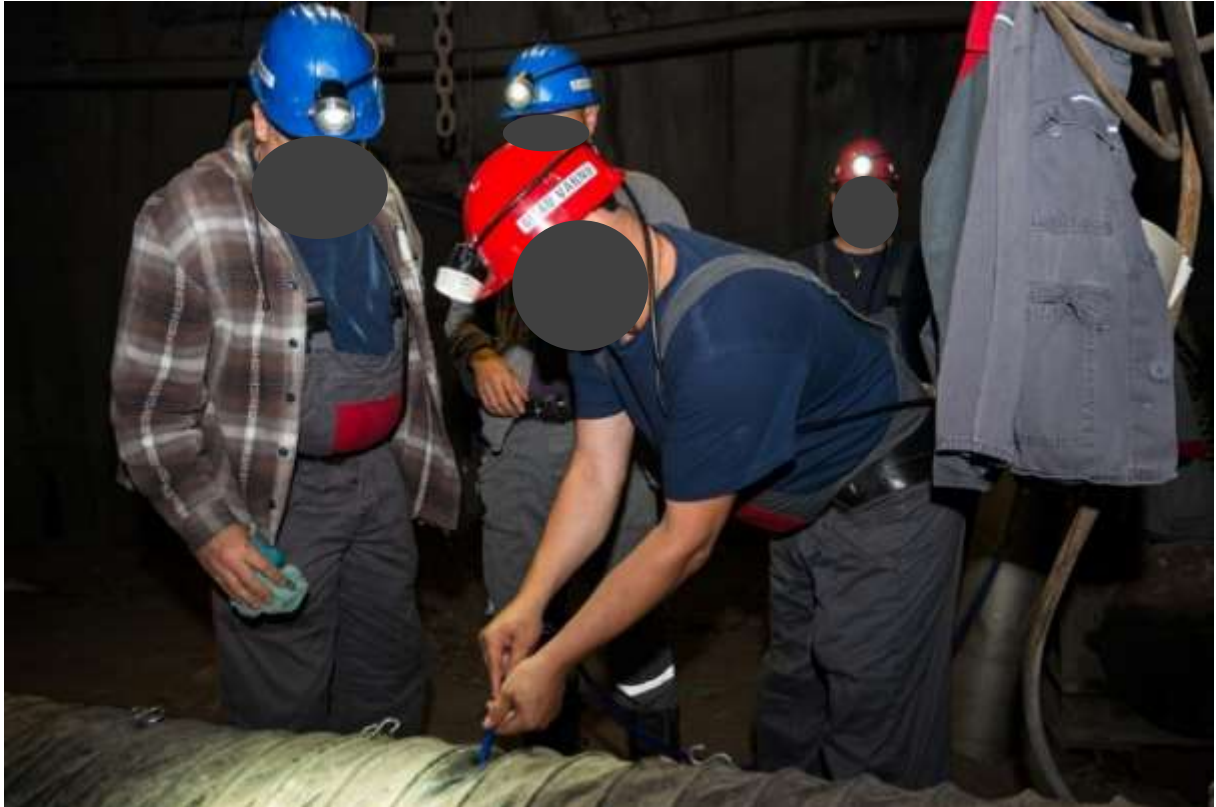
Figure 3.18: Inserting the tube connected to the DMS cylinder into the duct approx. 10 m before the DMS sensor on location 1 with respect to the flow direction.
