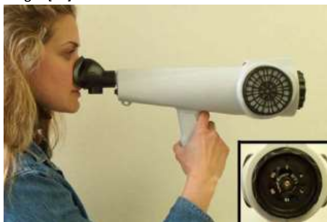
Figure 5.12: The Nasal Ranger Field Olfactometer [22]. The inset picture shows a close-up of the orifice dial, which is located in front Nasal Ranger ® .
