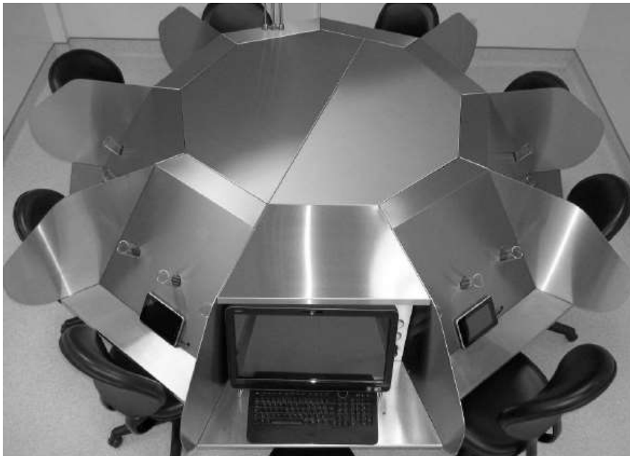
Figure 5.10: Design of a 9-sided (nonagon) ONOSE-8 ® stationary dynamic olfactometer operated at Consumaj laboratories in Canada. Allows simultaneous olfactometric analyses for 8 panel members, which significantly reduces the duration of the analysis. It meets all requirements of the CEN odour testing standard, EN13725:2003 and ASTM International E679-04. [141].
