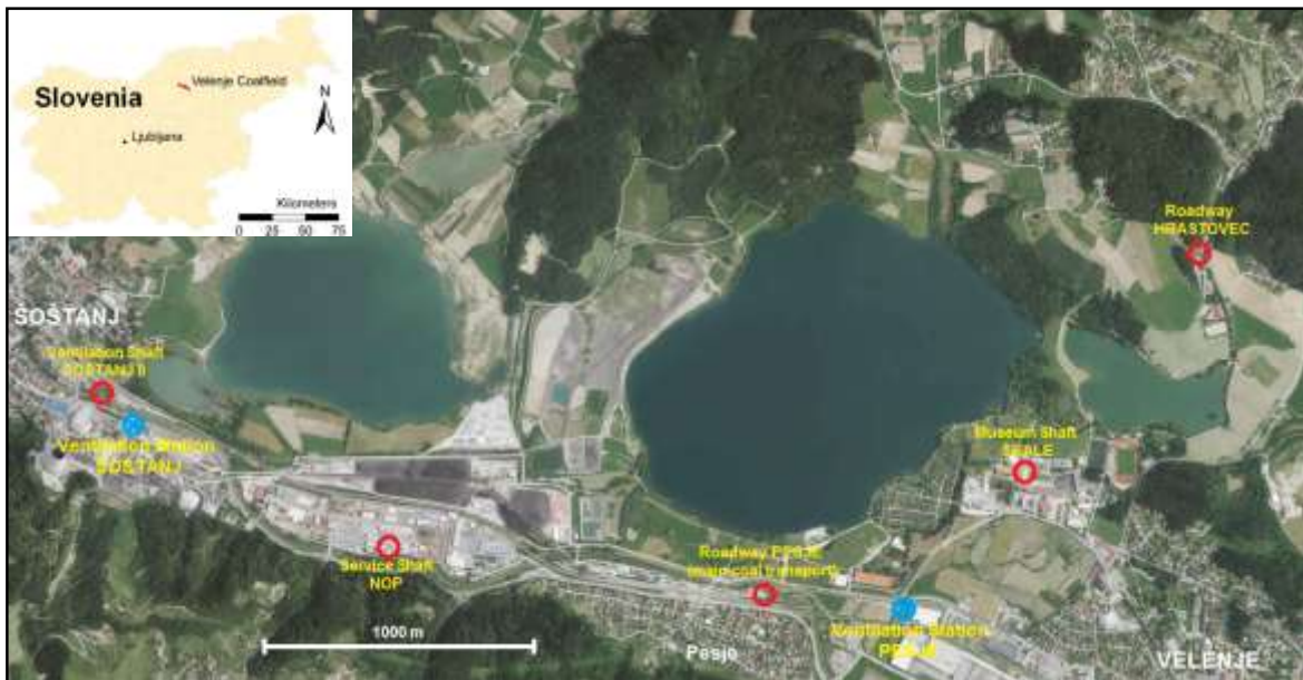
Figure 1.2: Geographic location of the Velenje Coal Basin. The two main fan stations (exhausting) are shown in blue and fresh air intakes are shown in red (situation in October 2012).
