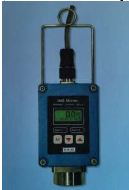
Figure 3.12: DMS sensor Type MONIMENT GMM 05.05
