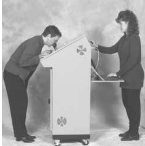
Figure 5.9: The AC'SCENT ® International Olfactometer was designed specifically to meet all requirements of the CEN odour testing standard, EN13725:2003 and ASTM International E679-04. [140].
