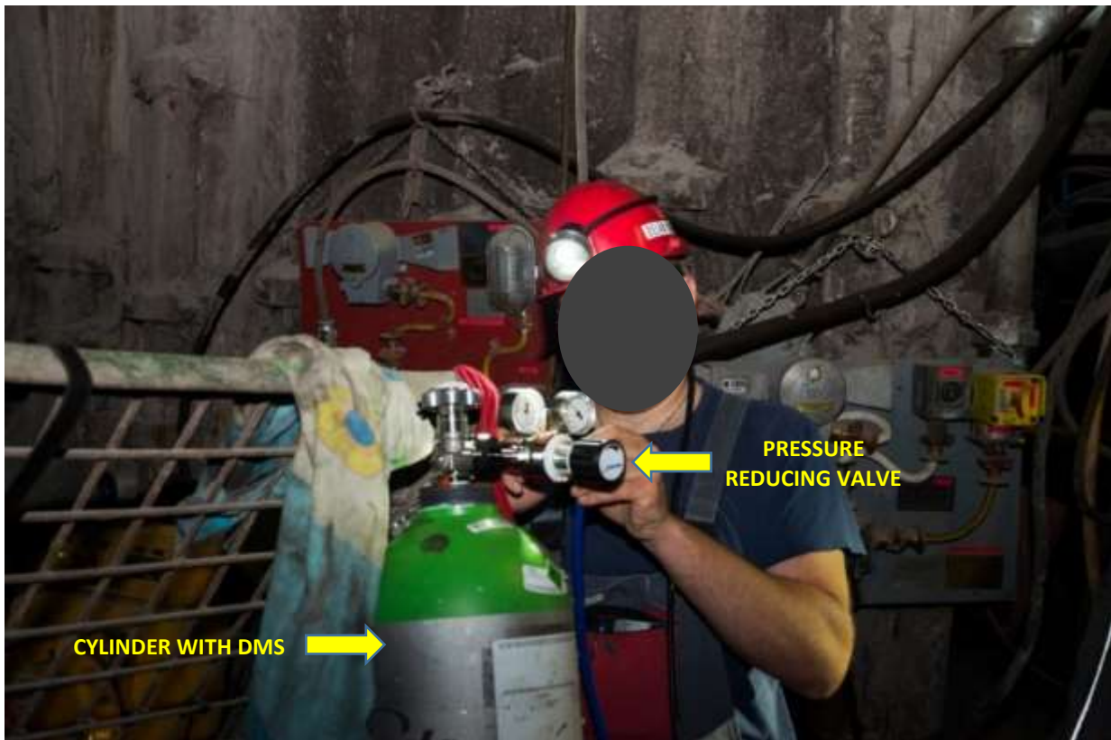
Figure 3.16: Preparation of a cylinder with DMS and a pressure reducing valve for flow regulation.
