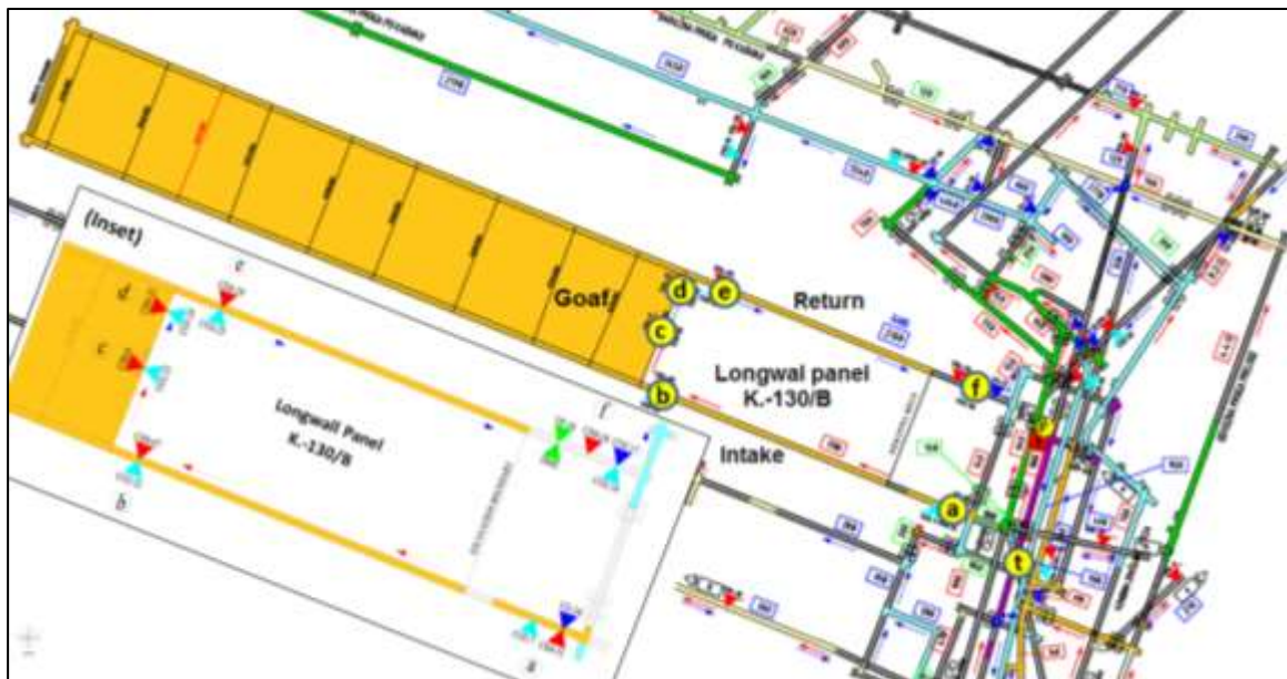
Figure 3.1: Longwall panel K.-130/B showing sensor positions a to f (in more detail on the inset) and the coal tonnage monitoring station t (longwall face as on 15 October 2012).
