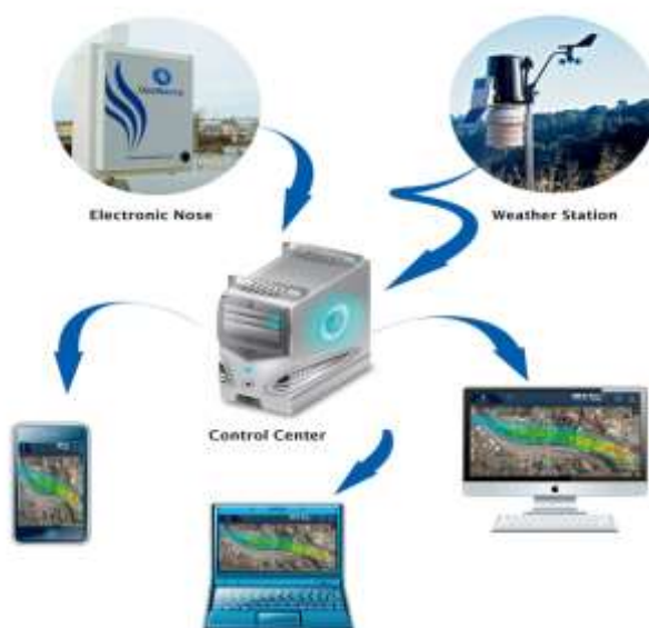
Figure 5.7: OdoWatch® – Odor Smart Monitoring : 24/7 odour measurement with eNoses, real-time odour plume dispersion modelling & automatic odour alerts [138].
