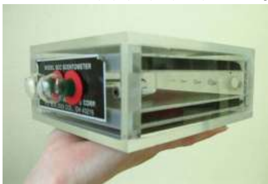
Figure 5.11: The Scentometer Field Olfactometer [22]. Note the two glass nostril ports to the left and the series of orifice holes at the back of the unit to the right in this photo.
