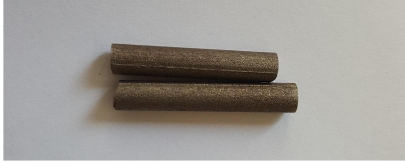
Figure 33: A test specimen of CVC NiTi rod before and after the 4-point bending test.
