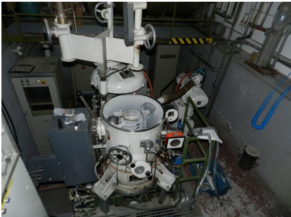
Figure 8: Vacuum Induction Furnace with mechanism for Continuous Casting.
