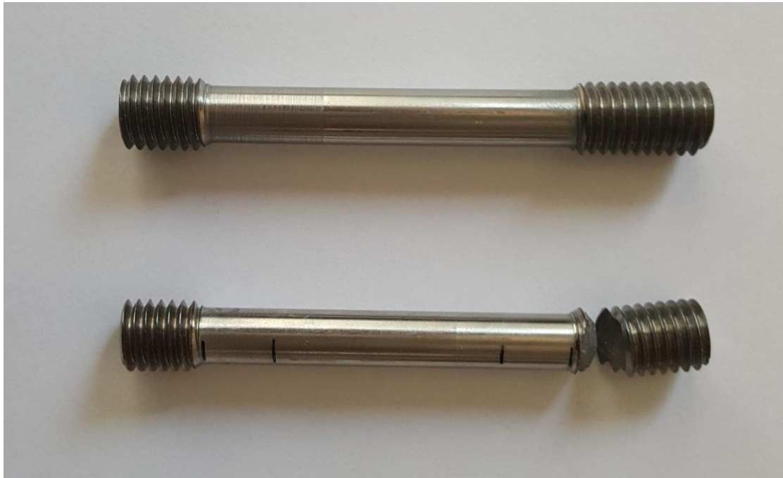
Figure 29: A test specimen of CVC NiTi rod before and after the tensile test.
