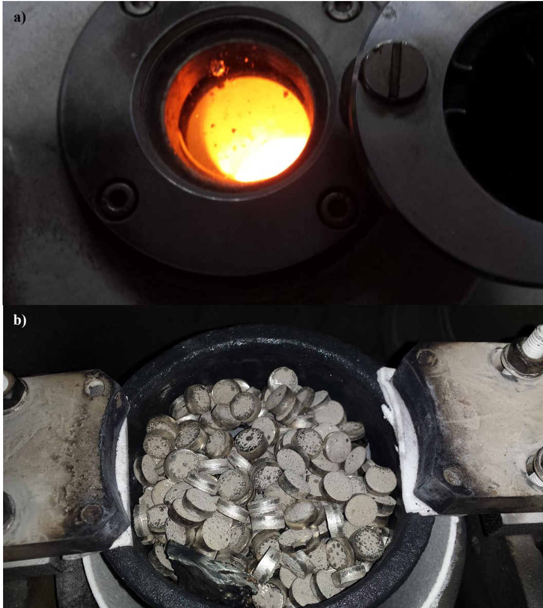
Figure 18: a) Clay-graphite crucible and b) the correct sequence of filling up from the walls to the middle of the crucible: Ti-Ni-Ti.
