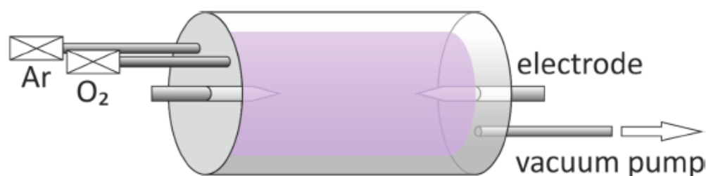
Figure 1. Schematic diagram of a custom-made plasma-enhanced horizontal tube furnace deposition system. The vacuum-sealed glass cylinder reactor has two electrodes with pointed ends from each side, and these two electrodes are used to ignite plasma.
