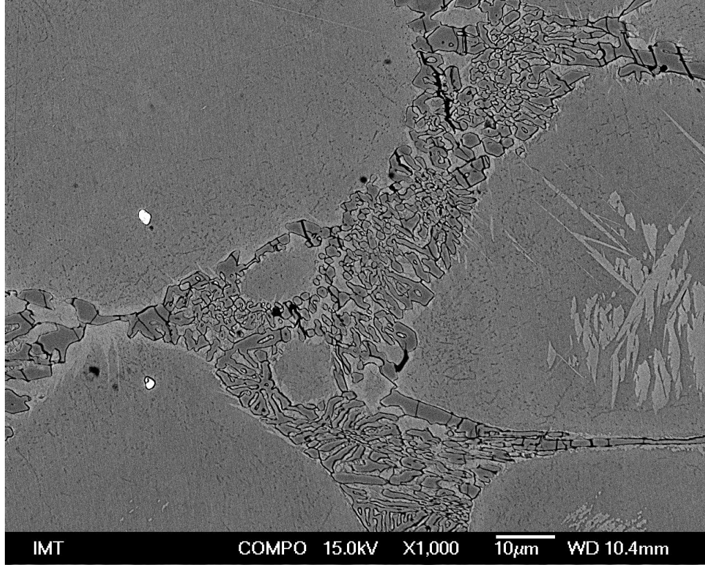
Figure 4.29: SEM BEI of microstructure of REE-modified AISI D2 tool steel on lower magnification. Bright spots on the figure represents REE containing non-metallic inclusions.
