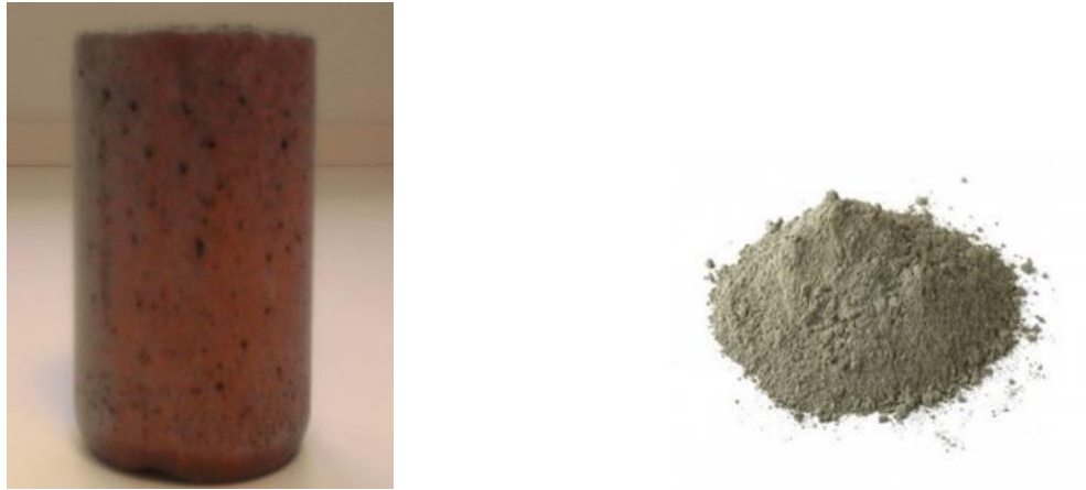
Figure 3.1: Compact and ground building composites.
