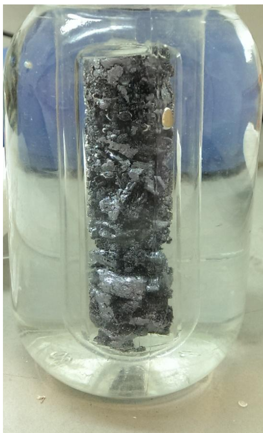
Figure 3.3: MoS 2 expanded in N 2 H 4 :H 2 O/NaOH solution at 60 °C. The reaction lasted for 24h.
