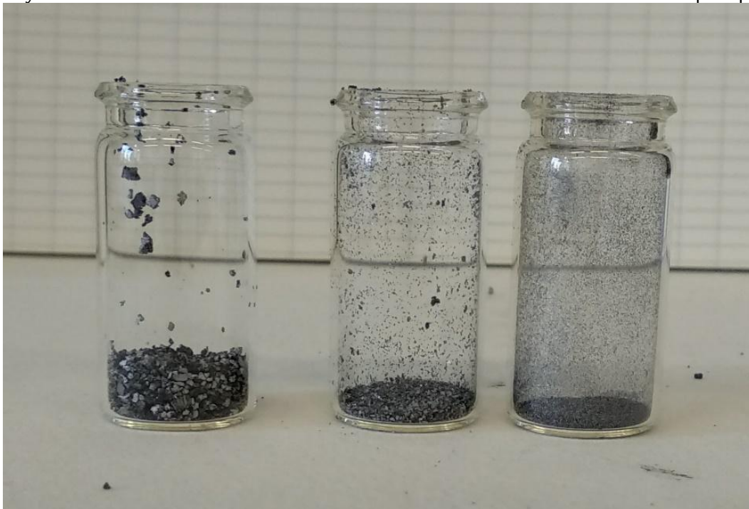
Figure 3.19: Comparison of expansion volumes of equal amounts of MoS 2 of different sizes (as in Figure 3.18): >300 \mu m (left), 300 \mu m>60 \mu m (center) and <60 \mu m (right).
