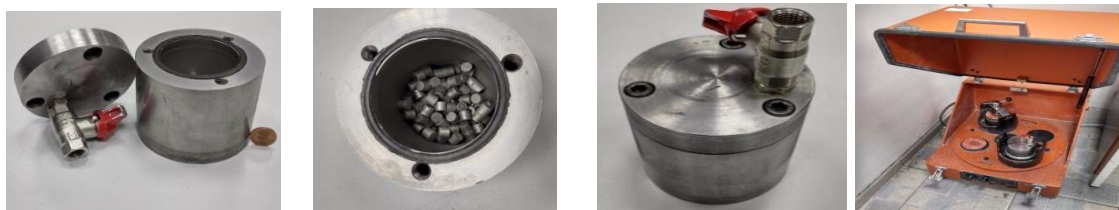
Figure 3.1: Scheme of decrepitation by rotating equipment; the magnets decrepitated are inside the jar to be put in the rotating equipment.
