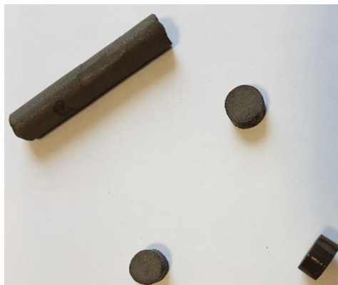
Figure 3.7: The Sm-Co polymer-bonded rods and final disc, the discs have a diameter of 1 cm.
