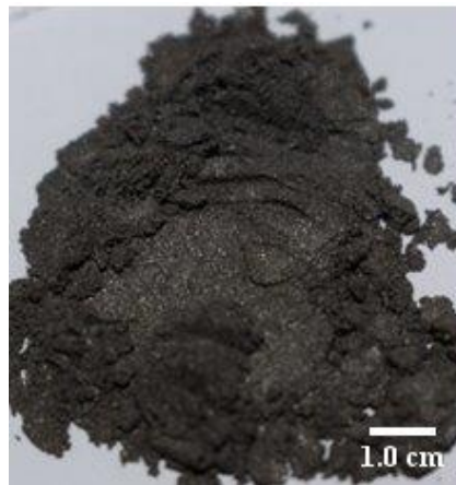
Figure 4.16: The decrepitated powder of coated SmCo 5 magnets using the rotating equipment. The coating material appears as silver particles imbedded in the magnet powder.
