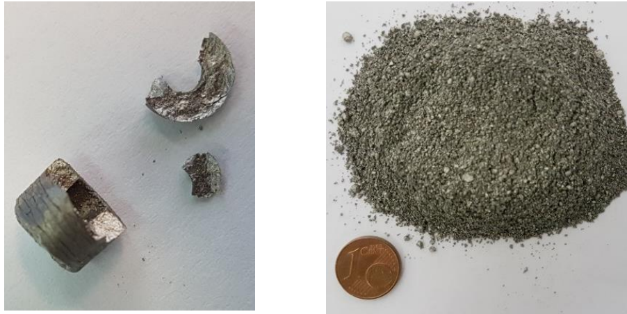
Figure 4.4: The fracture in the magnet structure due to the hydrogen absorption (left – scale bar for similar magnets in Table 3.1), and the decrepitated powders by using the stationary equipment (right).
