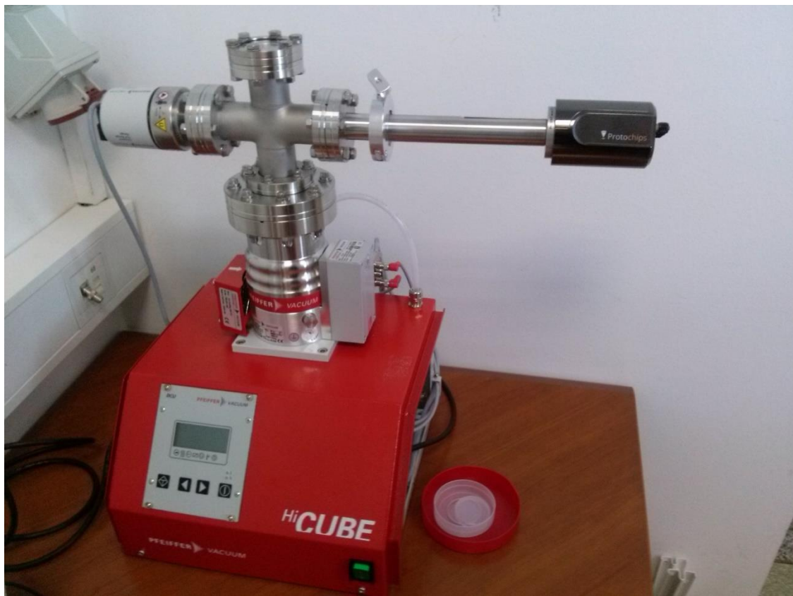
Figure 3.9: LCTEM heating holder performing a leak check.
