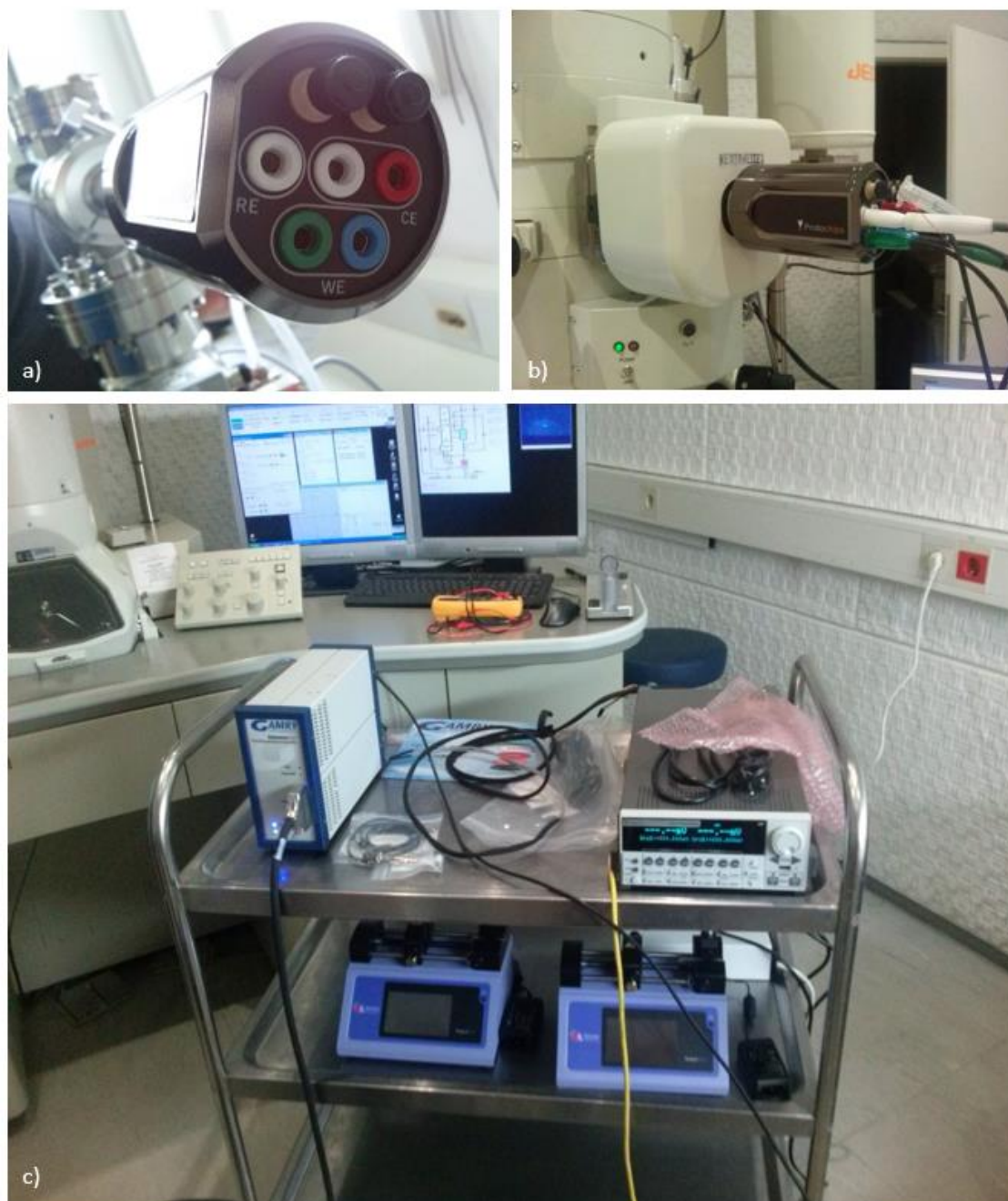
Figure 3.5: In situ electrochemical holder with two closed ports for liquid intake/outtake and ports for attaching the RE, CE, and WE electrodes. b) holder inserted in TEM c) Whole experimental setup with TEM, Gamry potentiostat and two syringe potentiostats.
