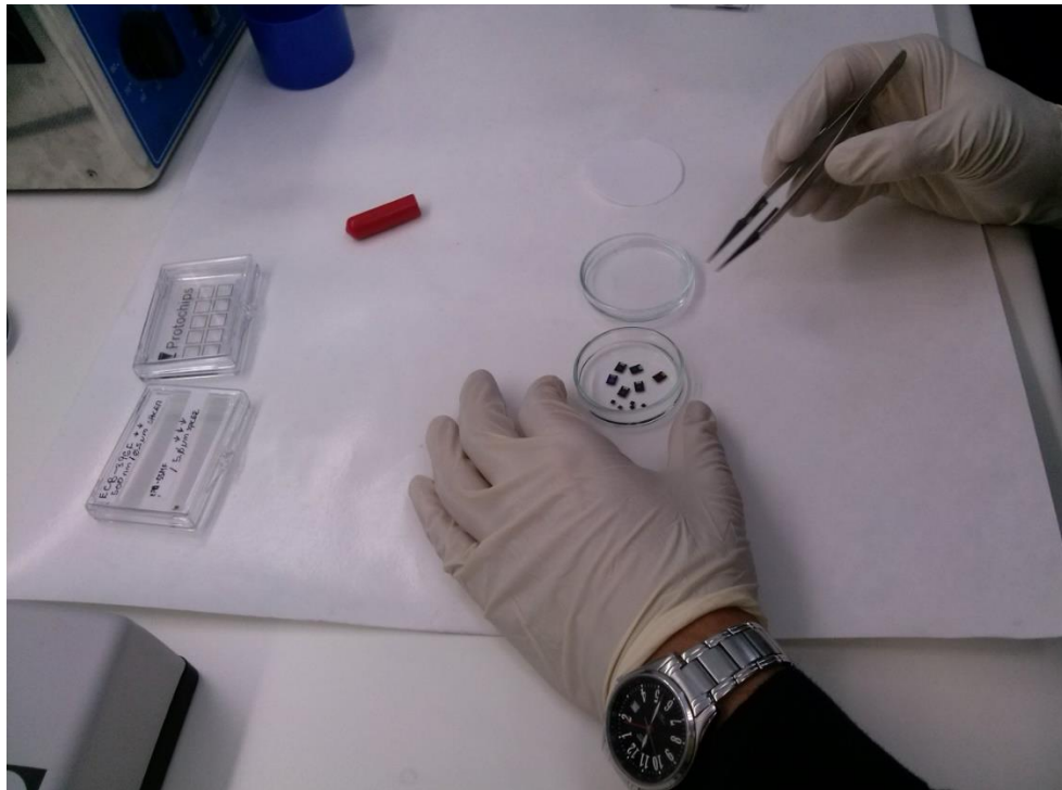
Figure 3.7: Initial cleaning of chips in a petri dish with an alcohol solution.
