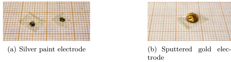
Figure 40: Reduced P(VDF-TrFE) copolymer films. Reduced P(VDF-TrFE) copolymer films with silver paint (a) and sputtered gold electrodes (b), prepared for dielectric measurements.
