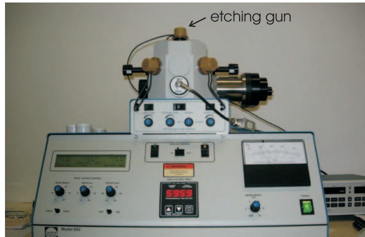
Figure 4.4: Gatan PECS system, which was used for ion beam sputtering of the bulk specimens.
