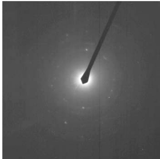
Figure 49: Diffraction pattern of the nanodroplet of Figure 48, where the crystal structure of the embryos is verified [104].
