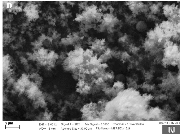
Figure 26: SEM images of particles deposited for (A): 30 min and (B): 2 h; (C): higher magnification of (B), (D): higher magnification of (C), some larger spherical particles of different sizes are indicated by arrows. For operational PLD parameters see also Figure 24.
