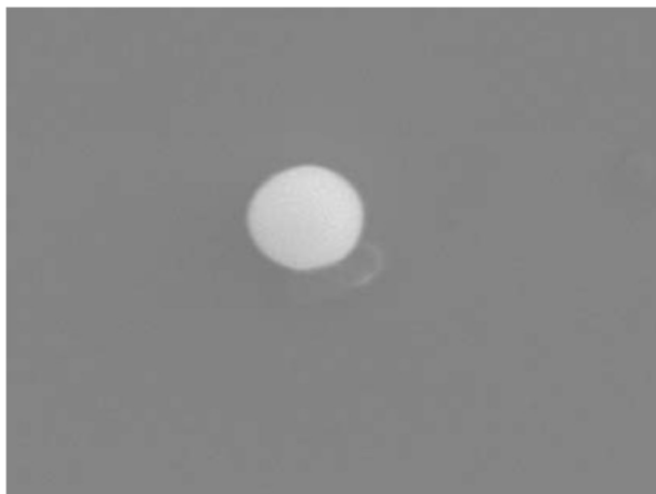
Figure 43: SEM image of a large size nanodroplet (500 nm diameter) [104].
