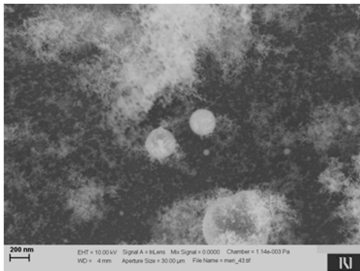
Figure 28: SEM image of particles with size distribution between 50 and 600 nm deposited on the substrate for 2 h.
