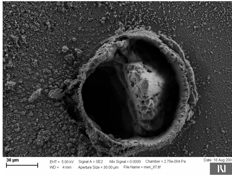
Figure 4: Splashing patterns on a \text{Sm}_{13.8}\text{Fe}_{82.2}\text{Ta}_{4.0} target.
