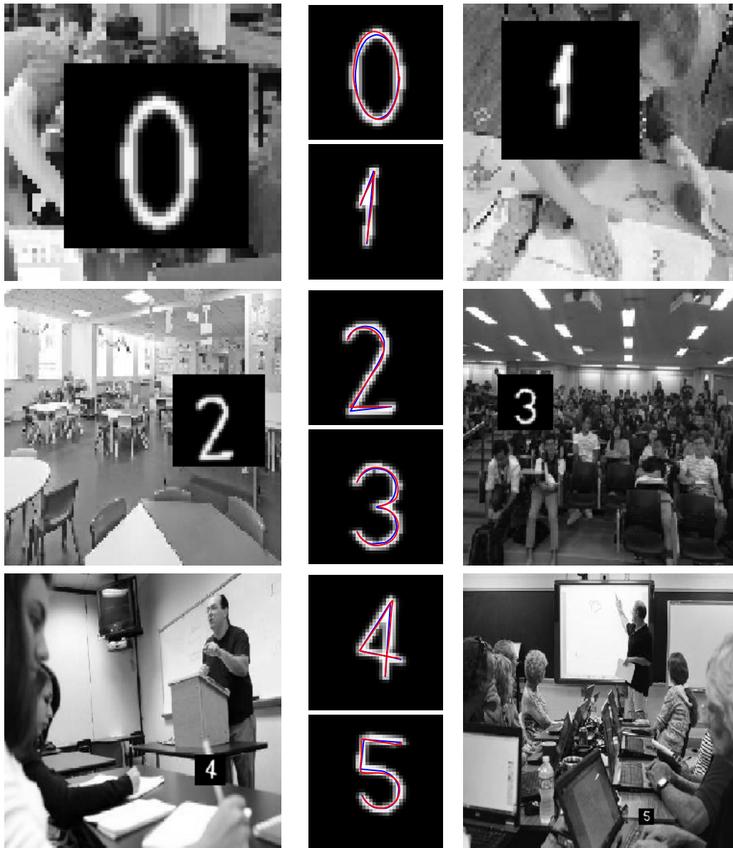
Figure 2.23: Visualization of writing trajectories generated by VIMEDNet trained with DMP trajectory loss function. The network can process images of different sizes at inputs. In this experiment, 40 \times 40 digit images were pasted onto 60 \times 60 , 80 \times 80 , 120 \times 120 , 200 \times 200 , 360 \times 360 and 680 \times 680 pixel background images. The neural network was trained with 80 \times 80 pixel images.
