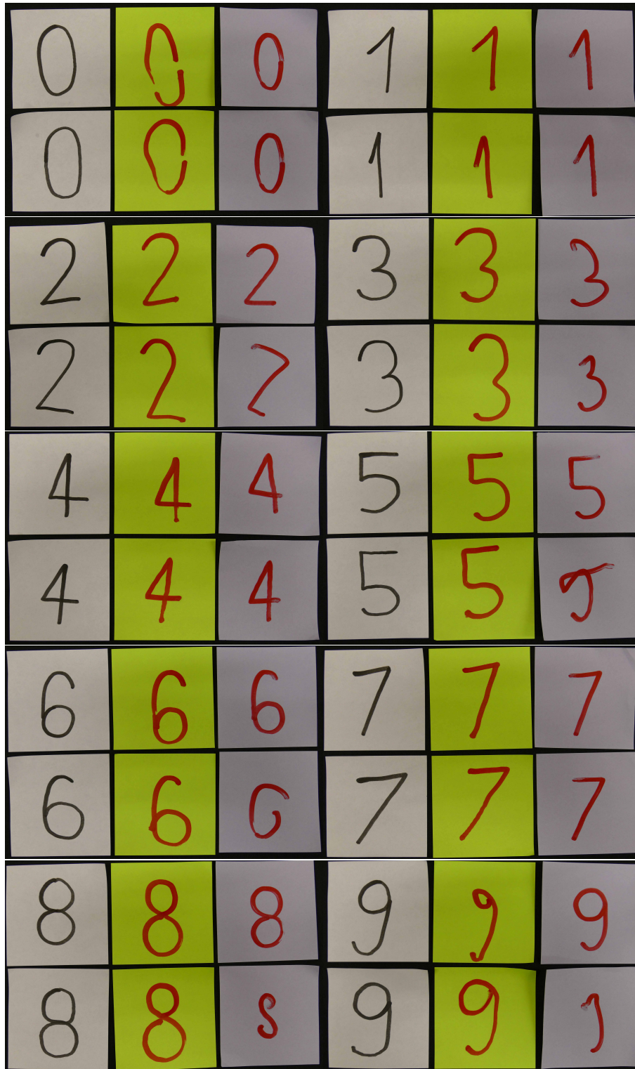
Figure 2.28: Digits written by TALOS using DMPs that were output by CIMEDNet and VIMEDNet. Red digits on yellow paper were generated using CIMEDNet, while red digits on grey paper were generated using VIMEDNet. Digits in black on white paper were handwritten by a human.
