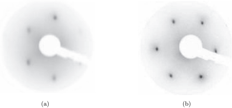
Figure 19: LEED diffraction patterns, recorded on a contaminated Cu(111) surface (a) and on a well ordered and clean Cu(111) surface (b).
