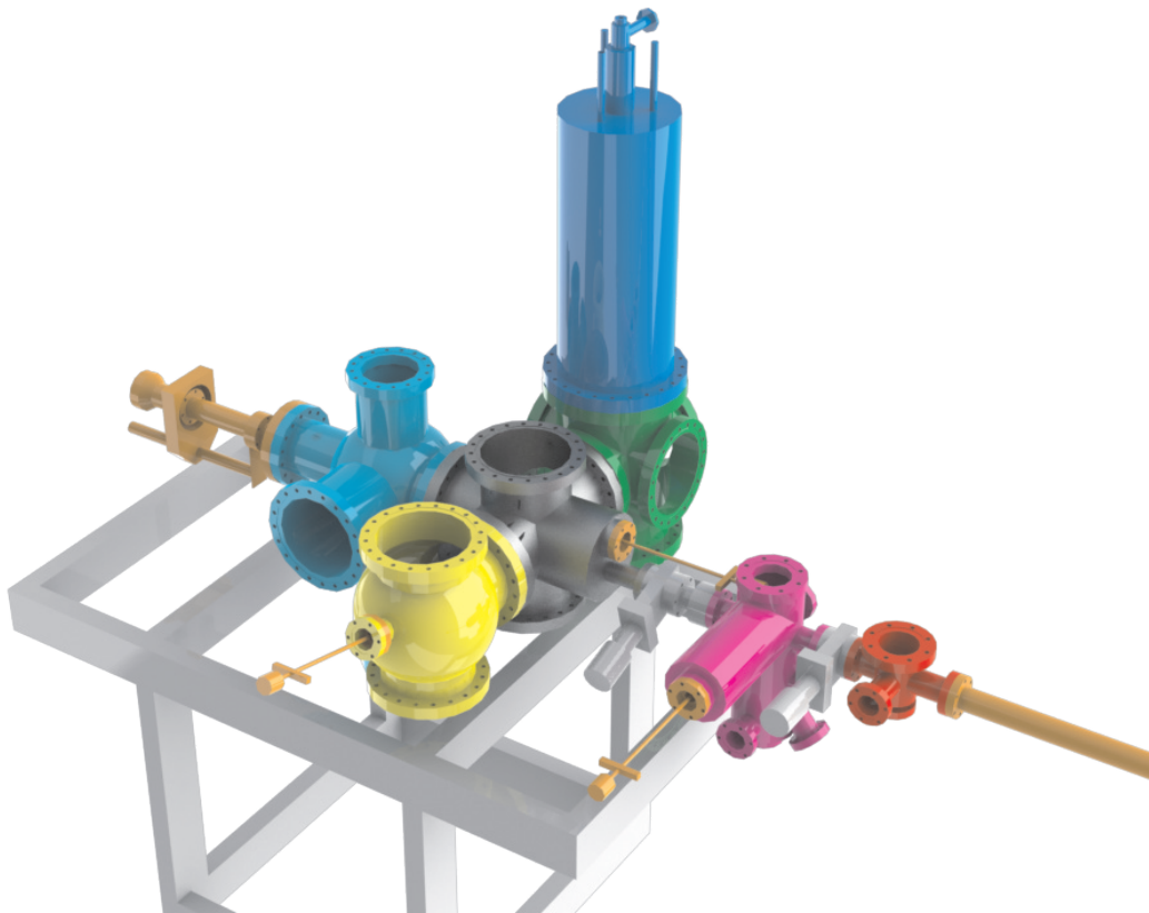
Figure 12: Schematic representation of the UHV system, consisting of a LT-STM chamber (green), a RT-STM chamber (yellow), a cryostat (blue), a sample storage chamber (gray), an analysis chamber (cyan), a preparation chamber (magenta) and a load lock (red).
