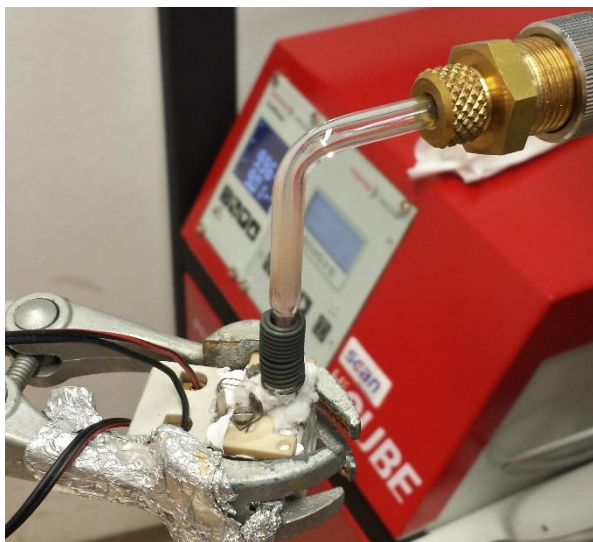
Figure 3.2: A heating cell with a sample (QMS). During analysis the cell is covered with the glass wool.
