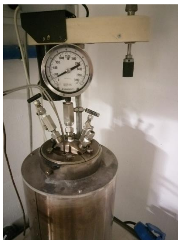
Figure 3.2: The autoclave used for the hydrothermal synthesis.
