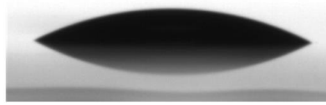
Figure B.3: Wettability measurements of a) plasma treated FTO and b) compact TiO 2 .
