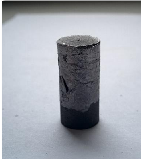
Figure 36: Graphite punch after processing the MQU-F powder at 800 °C.
