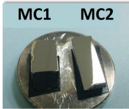
Figure 56: Polished cross-sections of the multicomponent magnets prepared from the raw powders (left) and pre-consolidated parts (right). The shining part on the right-hand side is an artifact due to the reflection of the illuminating spots.
