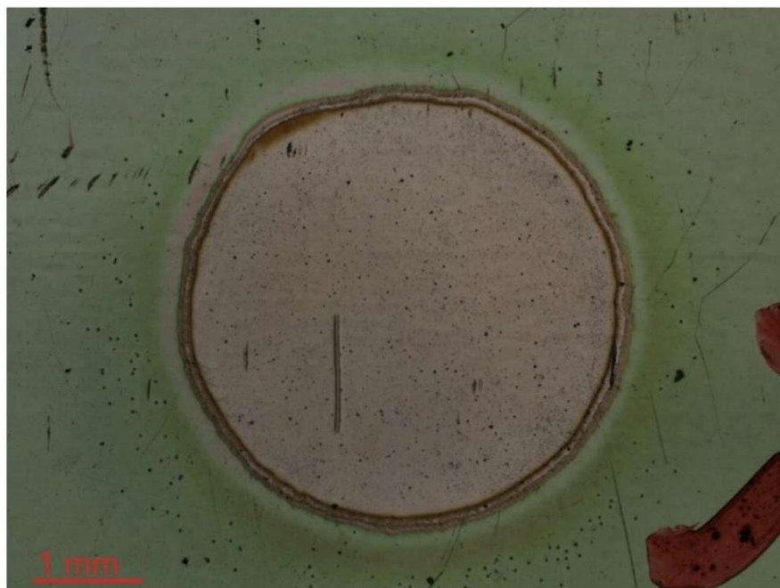
Figure S1. Bottom of the crater of the GDOES depth profile across a polymer film of thickness 500 nm using pure Ar.
